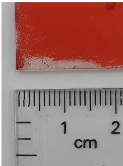
Figure 4.19. Damage on a gDR1 azobenzene thin film after curing at  $120^{\circ}\text{C}$  for 30 minutes.
